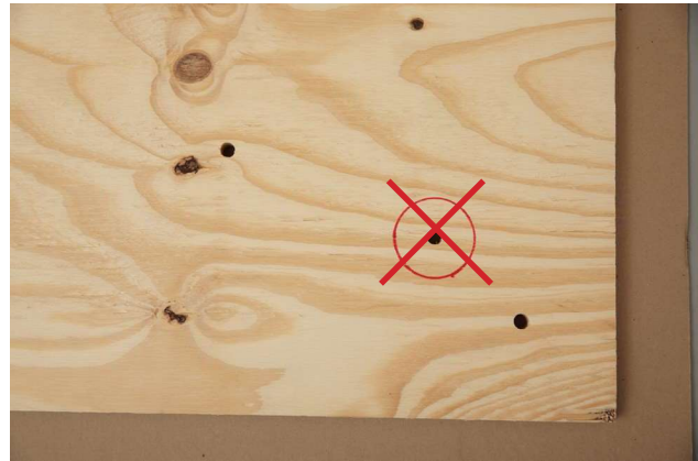
DO NOT INSTALL T-NUTS INTO HOLES WITH A CIRCLE
